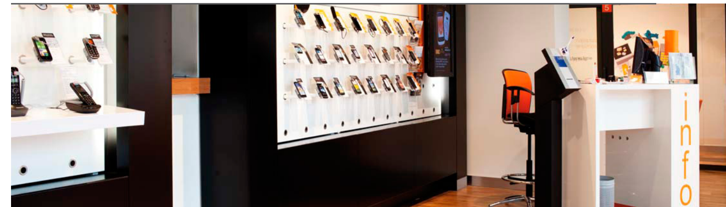
Display panels made of MDF on a metal structure together with holders for accessories made of polished stainless steel.
